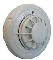
Thermovelocimetric detector consi-sting of a double thermistor. Interven-tion at  $58\,^\circ$  C. Prepared for testing by laser remote control. Alarm display LED. Output for alarm repetition. Pos-sibility of addressing via additional module. CPR certificate according to EN54 regulation part 5. Power supply 8-30Vcc. Operating temperature from - 20 to + 60  $^\circ$  C. Relative humidity up to 95% without condensation.
