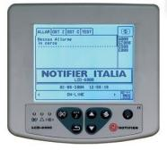
Repeating remote panel for addres-sed control units of the AM series. Graphic LCD display 320 x 240. It al-lows the recognition of the alarm and also the acknowledgment of outputs and the reset of the alarms with code complying with EN54-2. Power supply 10-30Vcc. Absorption at rest of 30mA and in alarm of 80mA. Dimensions: 180 x 168 x 55.
