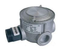
Propane detector in ADPE container. The catalytic type sensor guarantees alarm signals via a 4-20 mA propor-tional output. Connectable on central units addressed through a specific module. Possible use with relay bo-ard on double threshold control panels with 10 mA pre-alarm and 20 mA alarm. Operating voltage 12-24VDC. Absorption 90 mA. Operating tempe-rature from -10 °C to +55 °C. Rela-tive humidity up to 90%. CESI ATEX certification for AD detectors.
